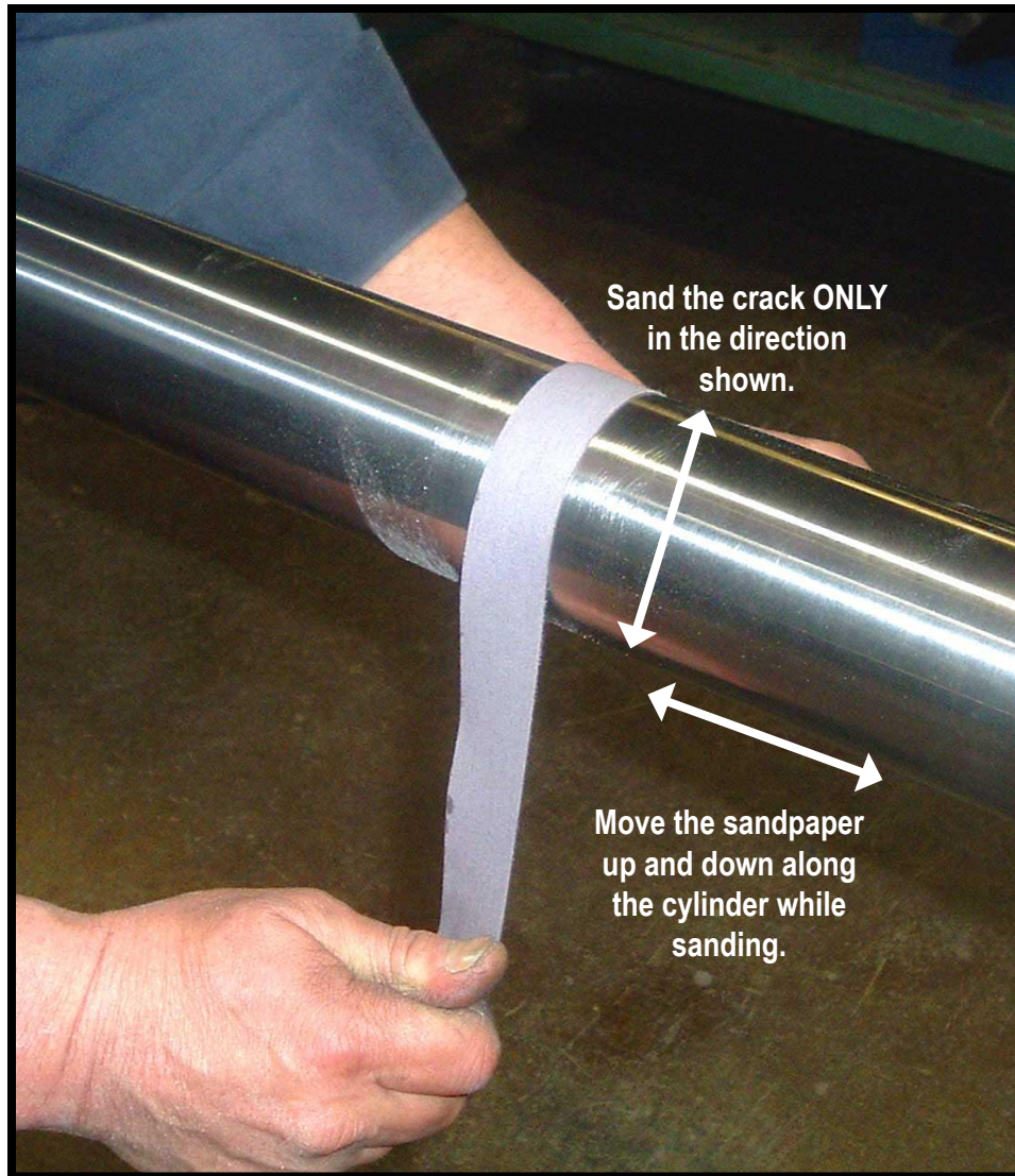
Figure 24 Split Cylinder Sanding
